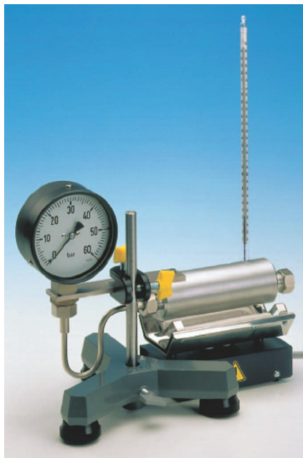
Fig. 1: Experimental set-up for measuring vapor pressure as a function of temperature.
