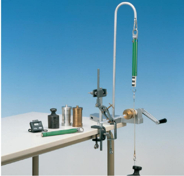
Fig. 1: Experimental set-up: Mechanical equivalent of heat.
